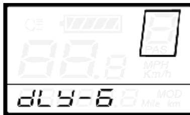
Delay time of battery power interface
